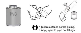
In Australia, you should use the Blue PVC glue. Green (which has greater strength) may be used if Blue is not available. Do not use Clear glue which is made for non pressure applications.
