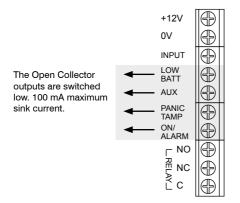
NOTE: The Open Collector outputs require no programming and are always active. The dipswitch settings mentioned in this manual apply only to the Relay Output.
