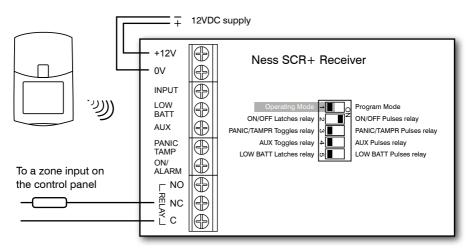
Note: For fully integrated radio operation on Ness control panels use the Ness 100-200 Radio Interface.
