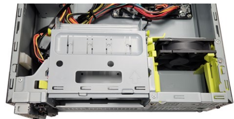
Quality hardware with 'Easy-Clip' storage carrier for easy installation of up to 2 x 3.5" optional hard drives.
