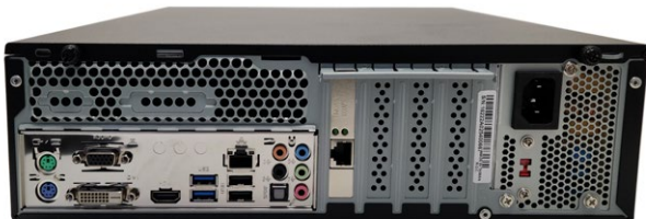
Multiple USB 3.0 ports, dual network ports, Multiple display outputs (displays usually only required for initial configuration of the server).
