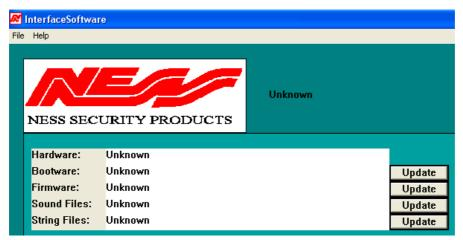
Once the utility program opens, if the RS232 cable is connected, it will attempt to connect to the Interface Module. (Note: If your PC does not have a RS232 port, you can use USB to RS232 leads such as the Ness 101-231 cable).
